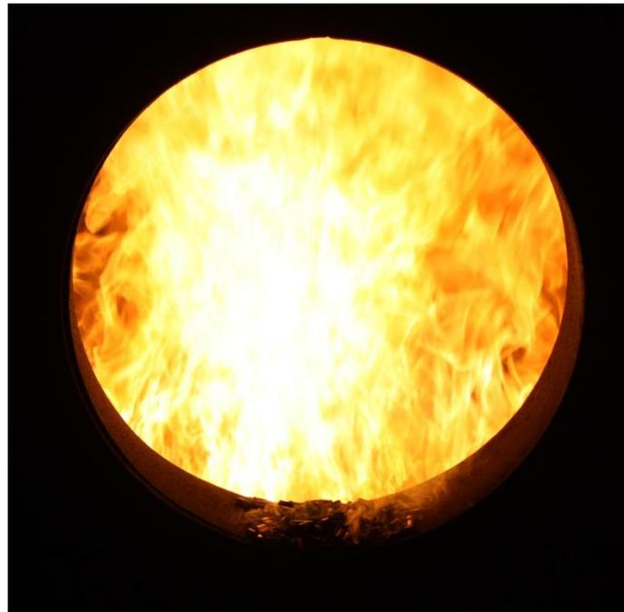
**FIGURE 5.** Burning straw pellets in the boiler furnace
